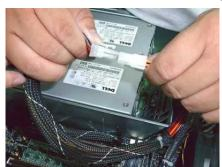
Connecting the PL-P3/SMP's power cable to the WTX power supply connector.
